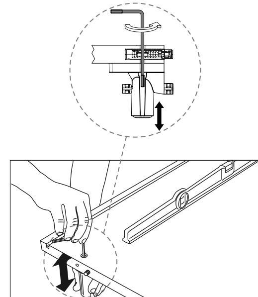
Height adjustment and check the level.
