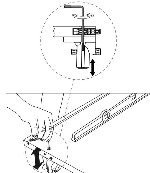
Height adjustment and check the level.
