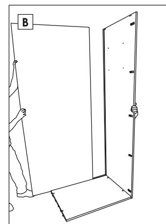
**Insert the back panel into base slot**
